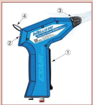
Pressing the full finger, short throw trigger (1) activates the static eliminating ions and airflow. Proper or improper functionality is indicated by a green or red LED (2). The non-marring nozzle (3) provides quiet performance and OSHA compliance. A hanger hook (4) is included to keep the Intellistat conveniently stored.
